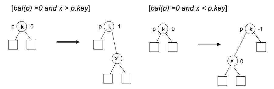
In both cases we need a procedure upin(p) which traces back the search path, checks the balance factors and carries out restructuring operations (so-called rotations or double rotations).
